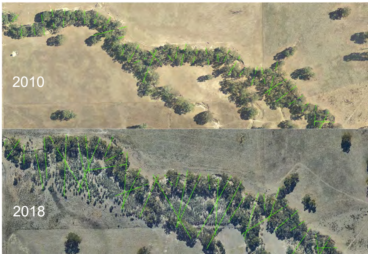
Figure 41 Histograms and aerial imagery showing vegetation width at Faithfuls Creek reach 21 in 2010 (Time 1) and 2018 (Time 2). The box at the top shows the % of sections where the vegetation width exceeds 10m, 20m and 40m in the two periods and the % change in the proportion of sections above those thresholds. Green lines on photographs are transects perpendicular to the stream used to measure vegetation width.
