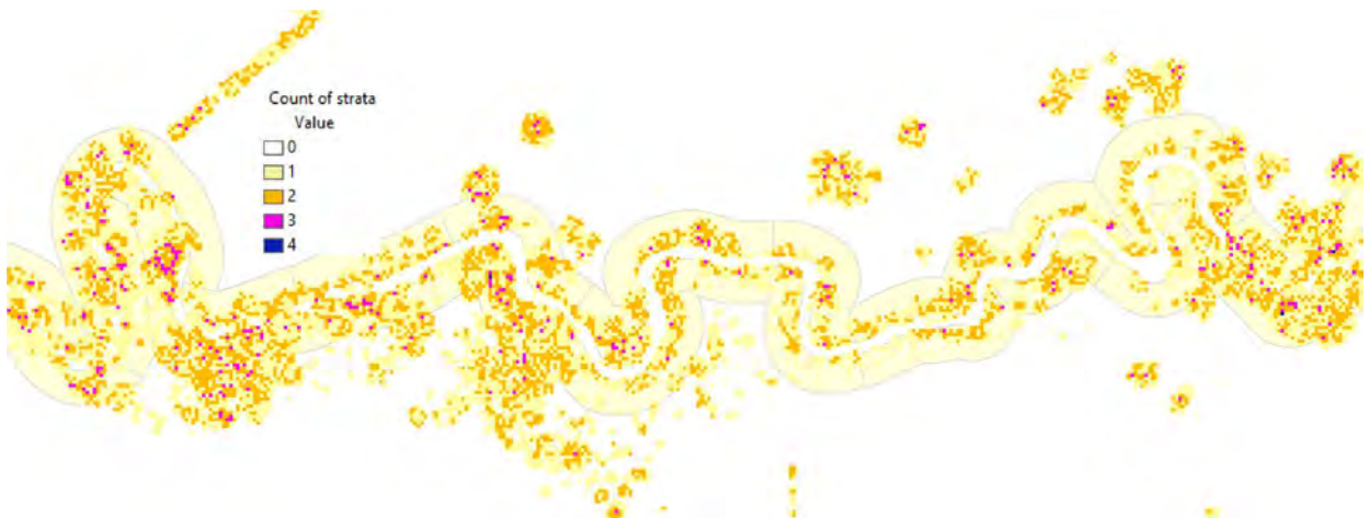
Figure 12 The Structure 2 metric is the count of 5m height classes present with FCC > 20%.
