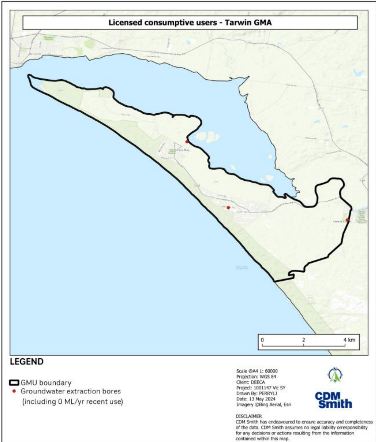
Figure X-36 Licenced groundwater extraction bores in watertable aquifers (consumptive users) within the Tarwin GMA
