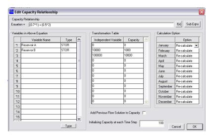
Figure 32 Capacity Information for Pipe Carrier from Reservoir A to Reservoir B
