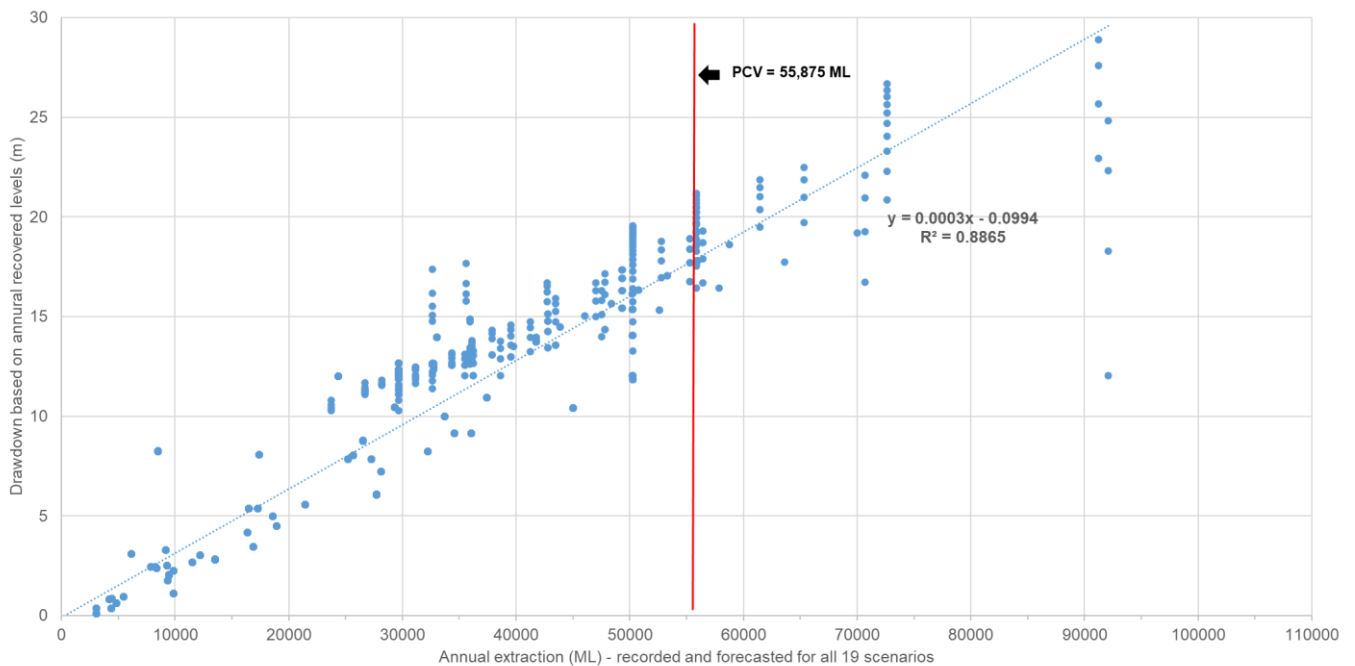
Figure 208 Lower Campaspe Valley WSPA Suite M_H_1: Drawdown (on annual recovered levels) and extraction volumes (recorded and forecasted <110,000 ML) for all data between 1972 to 2041 and all forecasted scenarios
