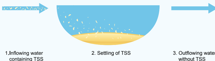
Figure 52: Schematic outlining how a sediment pond works with (1) water entering the pond, (2) water slowing and coarse sediment settling in the pond due to gravity. The water without TSS is on top and, finally, (3) flows out of the pond.
