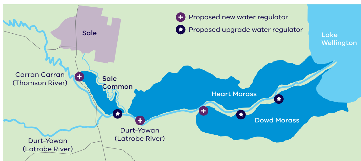
Figure 8.9: Proposed new and upgraded water regulating structures in the lower Latrobe wetlands
