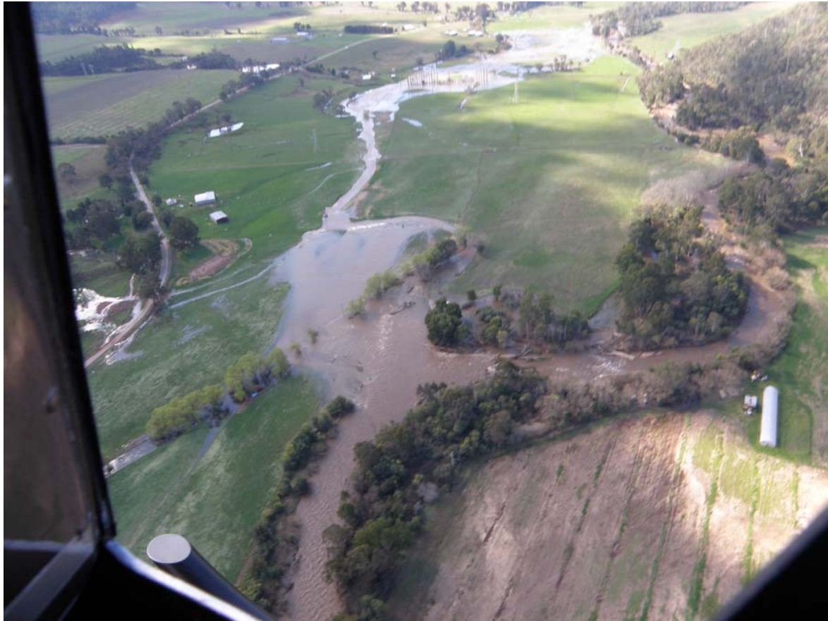
Figure 5. Floodplain flow and site of potential avulsion of King River in north east Victoria (View looking downstream, King River is on the right, floodplain scour path is in centre of image)
