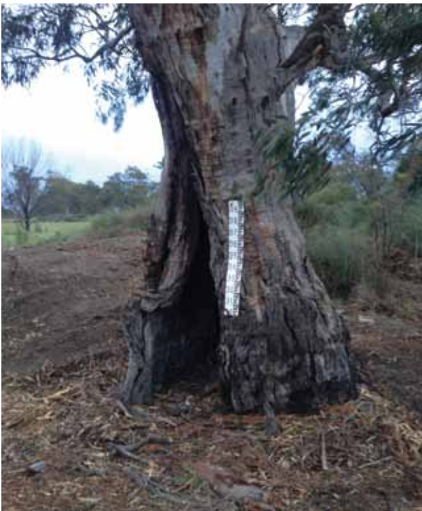
Flow depth gauge board at Benjaroop. Photo. Rohan Oliver, Ventia
