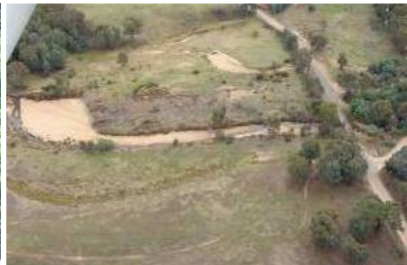
Stream bed aggradation, Reedy Creek, north east Victoria
