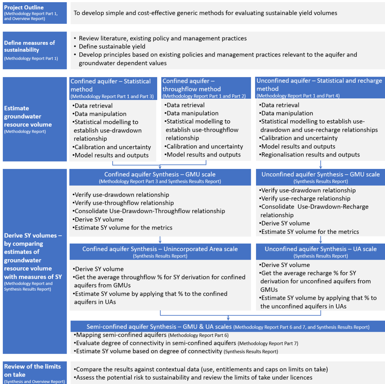
Figure 1. Synthesis flowchart for confined and unconfined outputs
