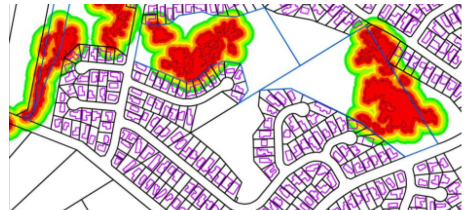
Figure 9 – Separation of the highest risk areas (Risk level A (red)) from buildings (purple), Little Bogy Creek Reserve, Frankston
