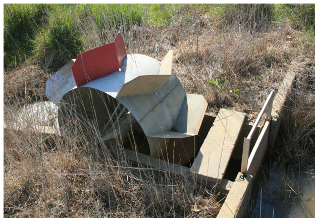
Irrigation dethridge wheel
