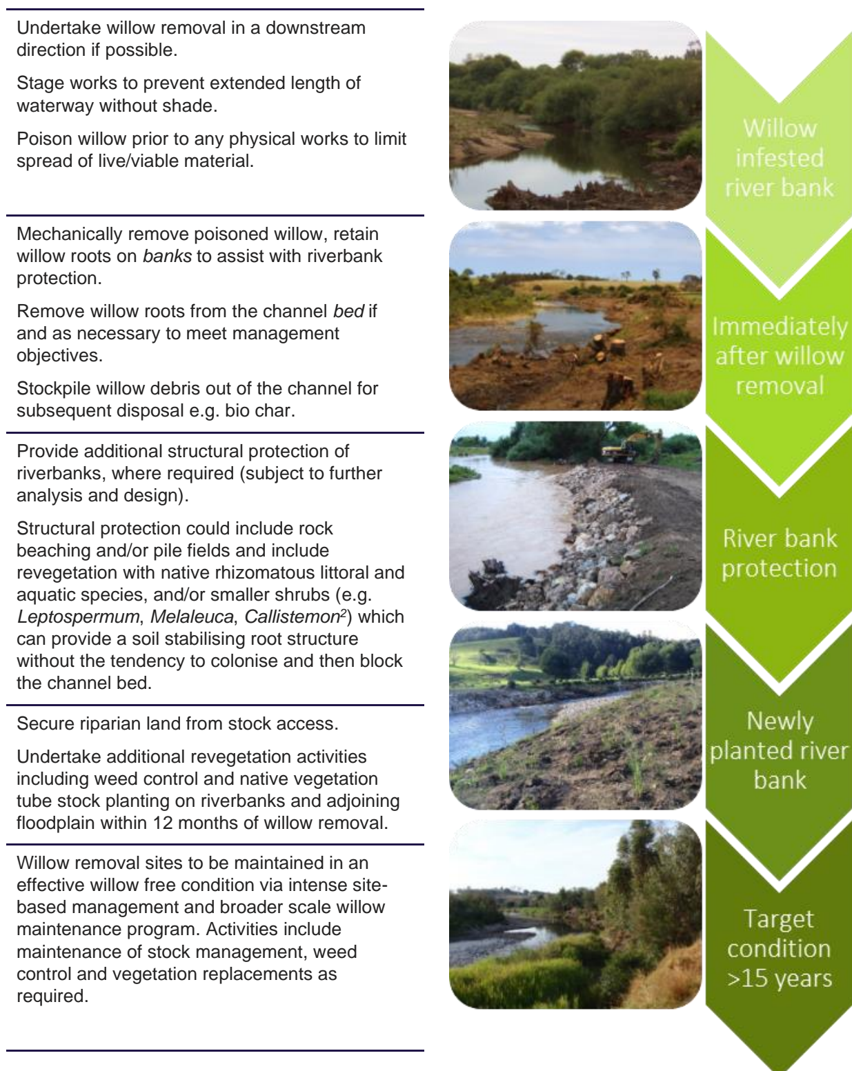
Figure 50. Approach for approach for willow replacement, management of willow debris and bank stabilisation.
