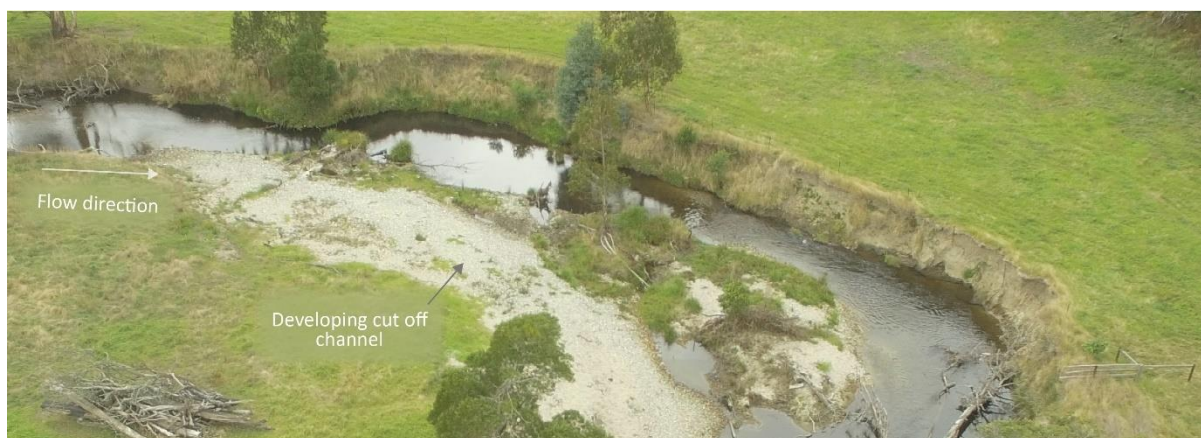
Figure 83. Example site meander bend showing bank erosion on outside of meander, and gravel point bar on inside meander on Errinundra River.
