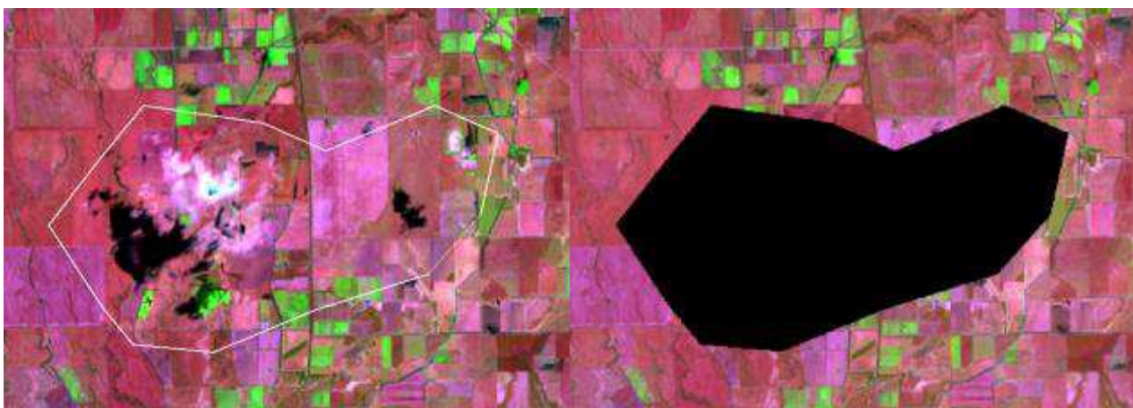
Figure 13. Landsat 8 image data from 18/4/2014 (path/row 94/85) with bands 5,4,2 in RGB (left) with vector in white outline overlaid over cloud affected area, and corresponding resultant cloud masked image (right) where the black area represent the masked out area.
