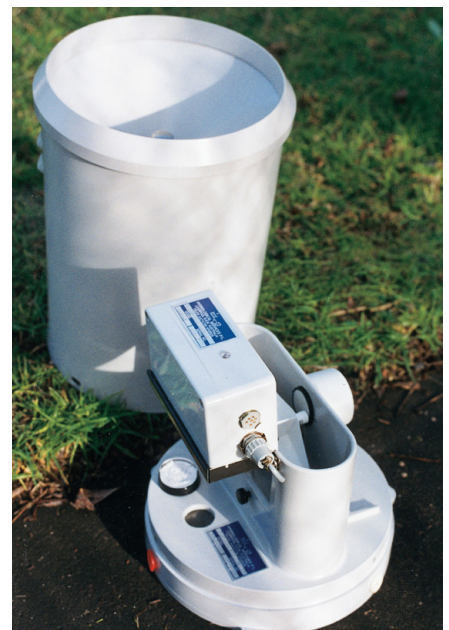
Photo: A tipping bucket rain gauge, data logger and funnel (instrument) / photograph by Mike Rosel. Copyright Commonwealth of Australia.
