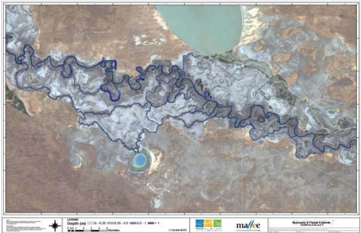
Figure 8-3-1. Modelled inundation extent of current conditions at Lindsay Island at flows of 40,000 ML/d (Water Technology, 2014)
