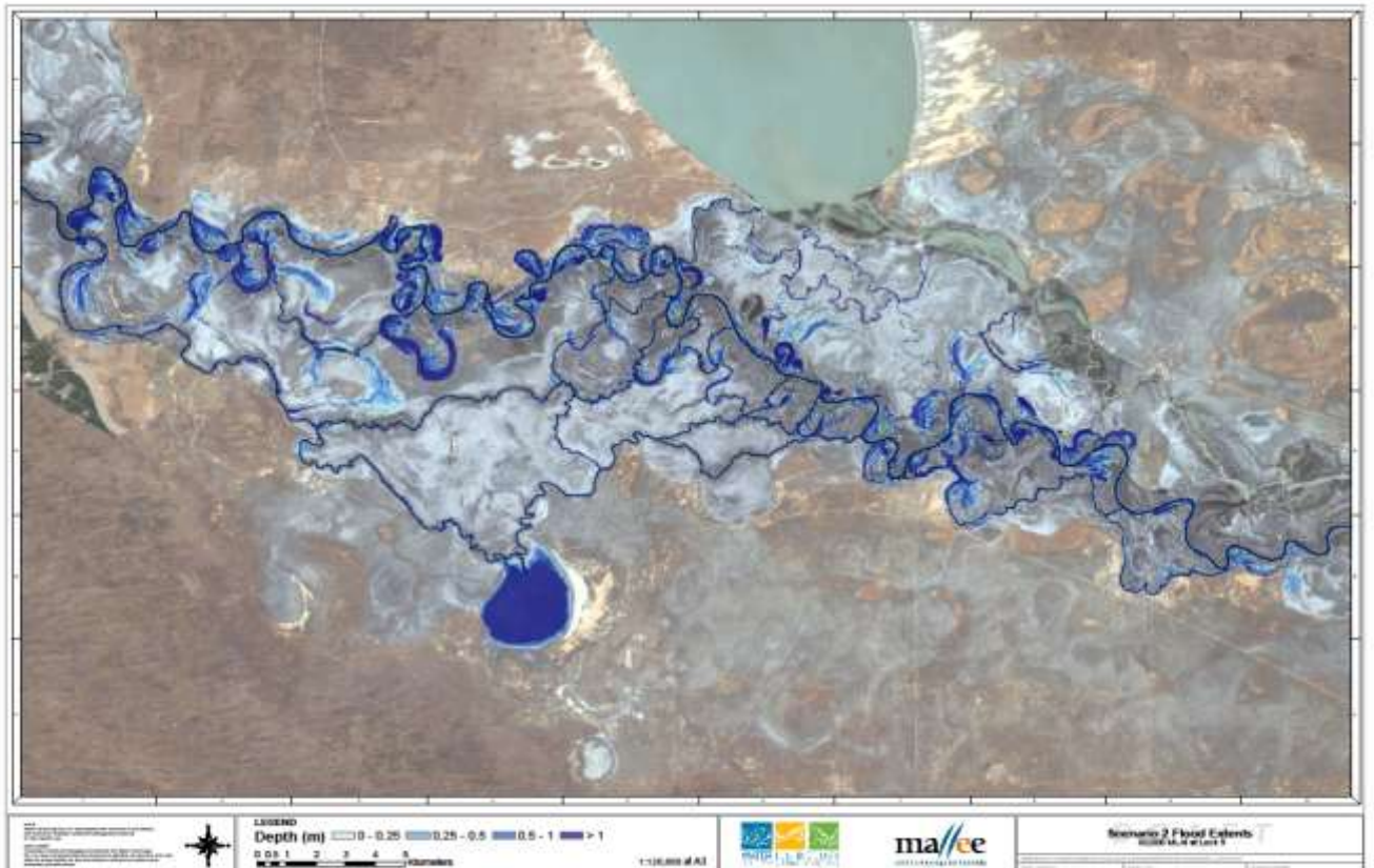
Figure 8-3-2 (above) and Figure 8-3-3 (below). Modelled inundation extent of current conditions at Lindsay Island at flows of 60,000 ML/d (above) and 80,000 ML/d (below) (Water Technology, 2014)
