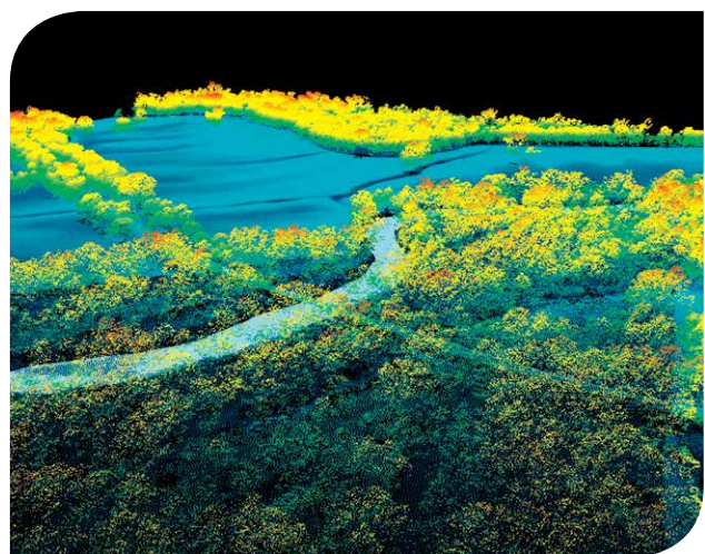
A 3D image of the ground surface showing vegetation generated using LiDAR technology. The different colours are due to the different height of the vegetation (red is taller). This image has not had the road and the bridge across the river removed.
