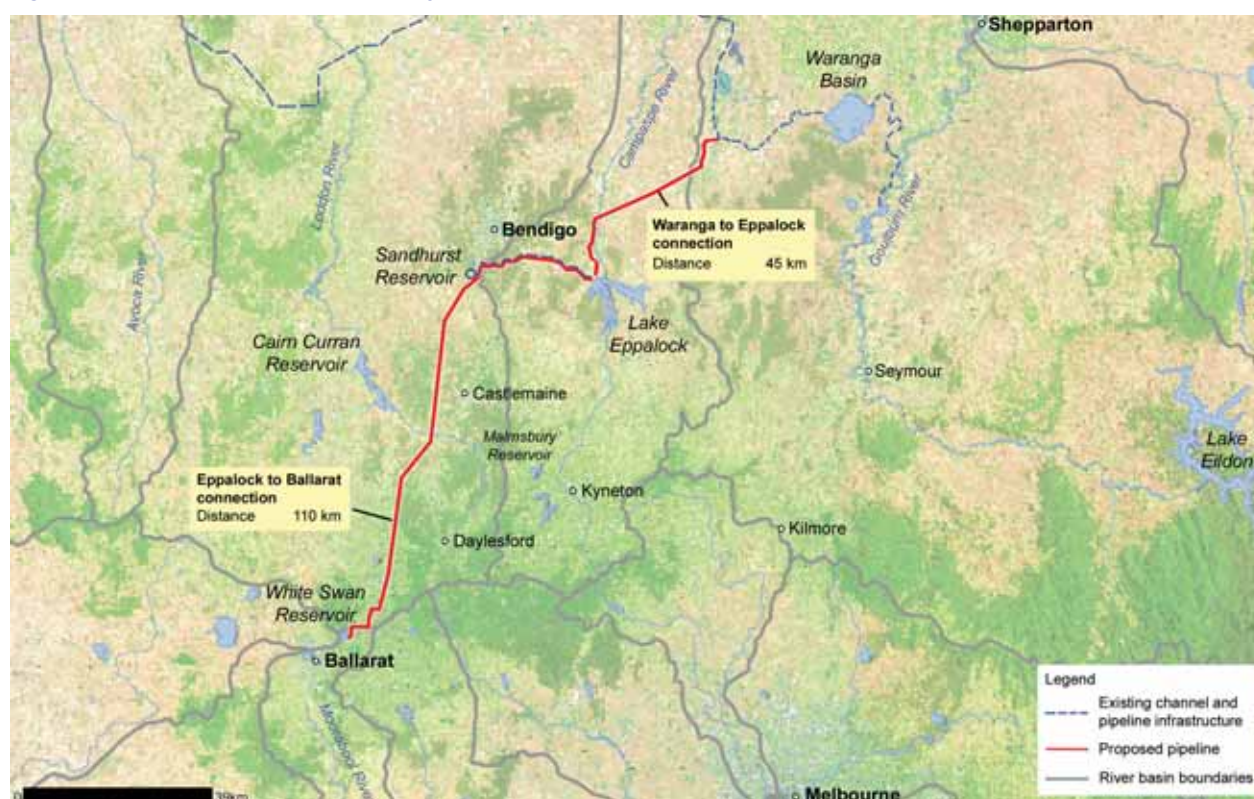
Figure 4.2 Connection from the Goulburn system to Ballarat
