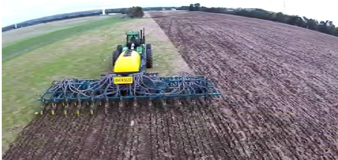
Figure 25. Zero tillage, direct-drill sowing into uncultivated pasture. Air-seeder points can penetrate the soil, place the seed and cover adjacent surface with soil. The pasture is likely to have been sprayed prior to sowing with a 'knock-down' herbicide to prevent pasture competition with the growing crop. Source: https://www.youtube.com/watch?v=YHqheE3NfMM .
