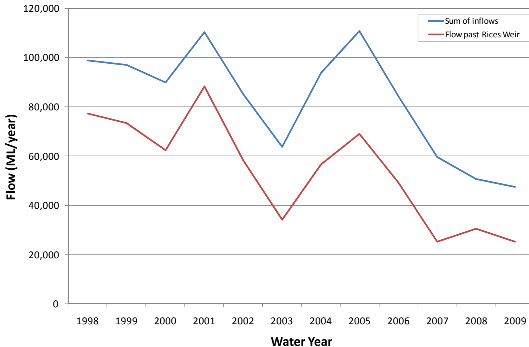
Figure 7-8 A comparison of annual total inflows (including from the upstream catchments, outfalls and drains) and annual flow past Rices Weir (some data infilled as outlined in Appendix D) up to 2009
