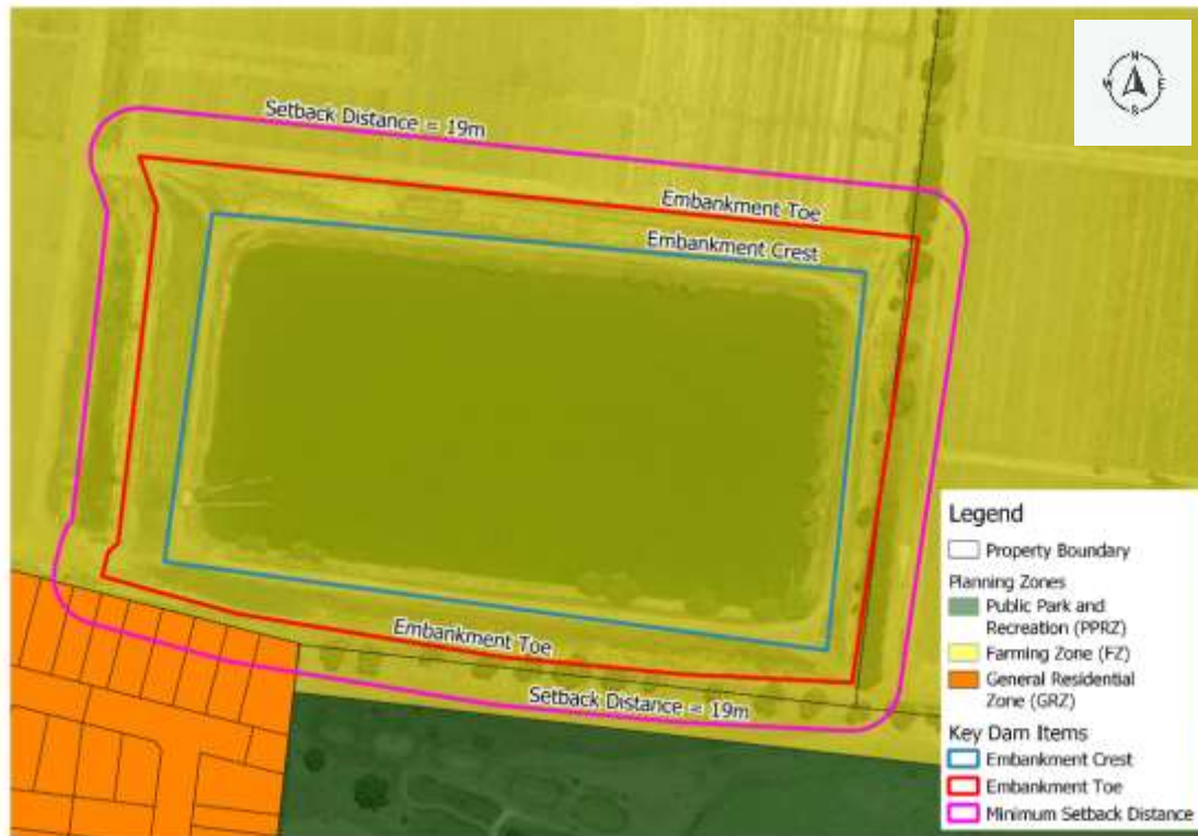
Figure 10: Example Calculated Minimum Setback Distance
