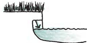
c. Slumping failure (slide → topple)
