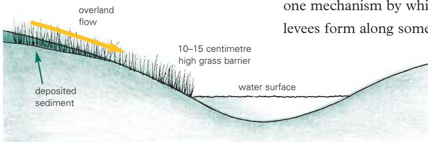
**How a grass filter strip functions to trap sediment.**
