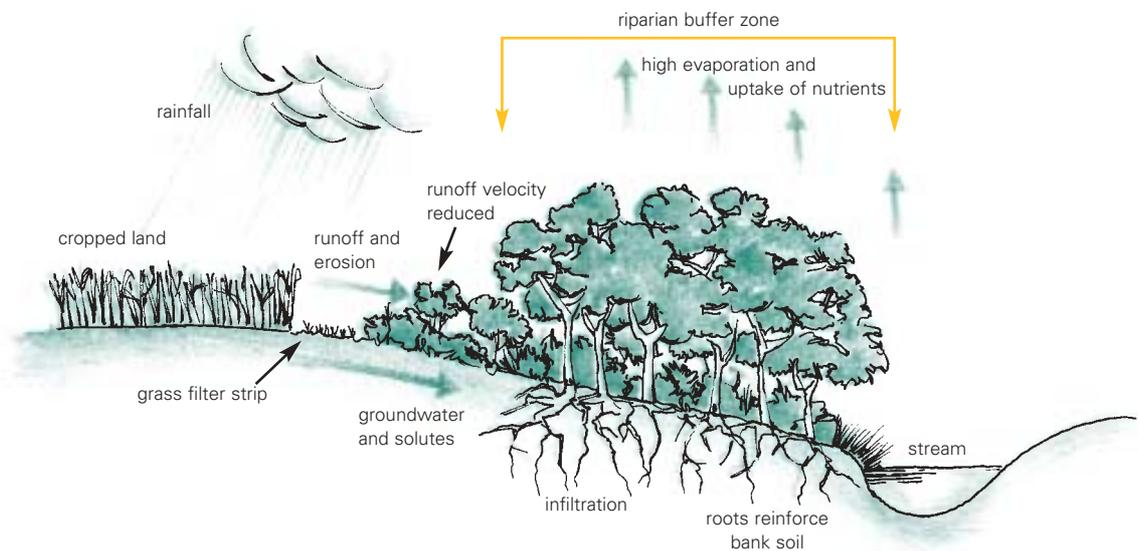
**How a riparian vegetation buffer and grass filter strip combine to trap sediment, nutrient and other contaminants.** Illustration The Idea to Here.
