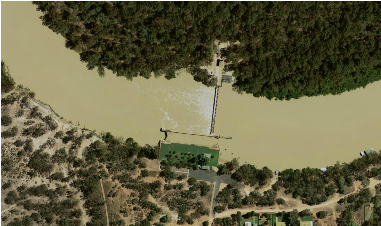
Figure 30. Lock 9 showing the lock on the south (left) bank. The fishway is on the north (right) bank. (Source: Google Maps)
