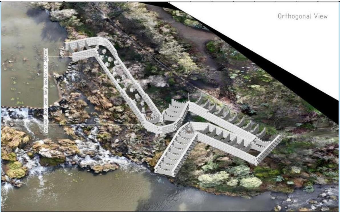
Figure 2: conceptual design of the fish ladder at Buckley Falls (supplied by CCMA)
