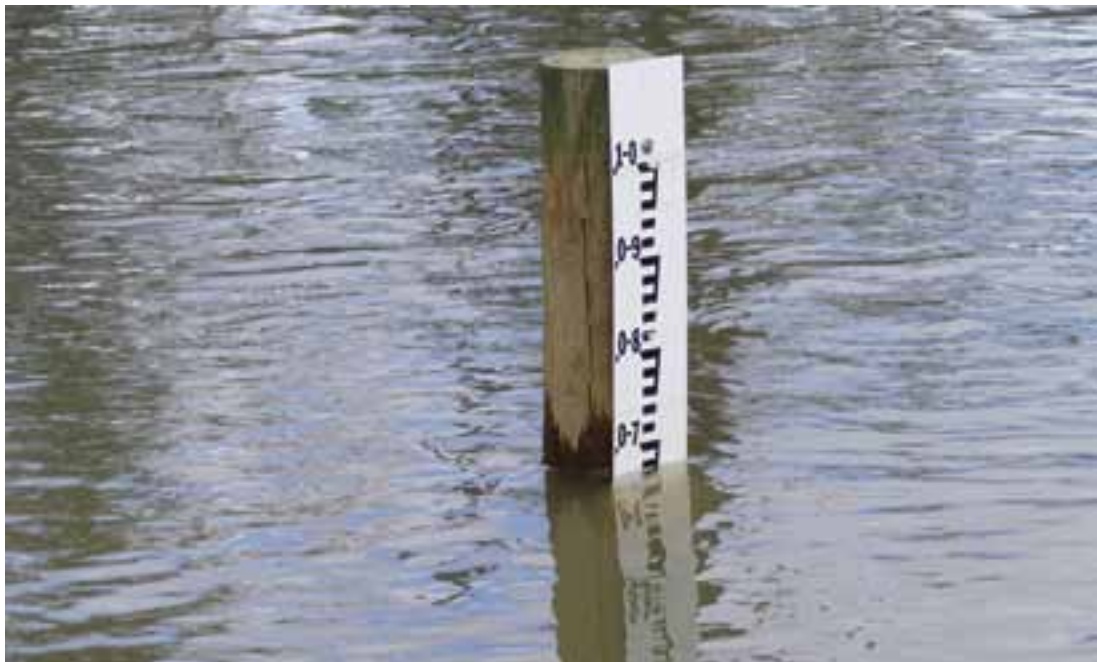
Figure 5.2: Gauge-board monitoring water depths during 2008 environmental flow release (Photo by Melanie Tranter, North Central CMA)
