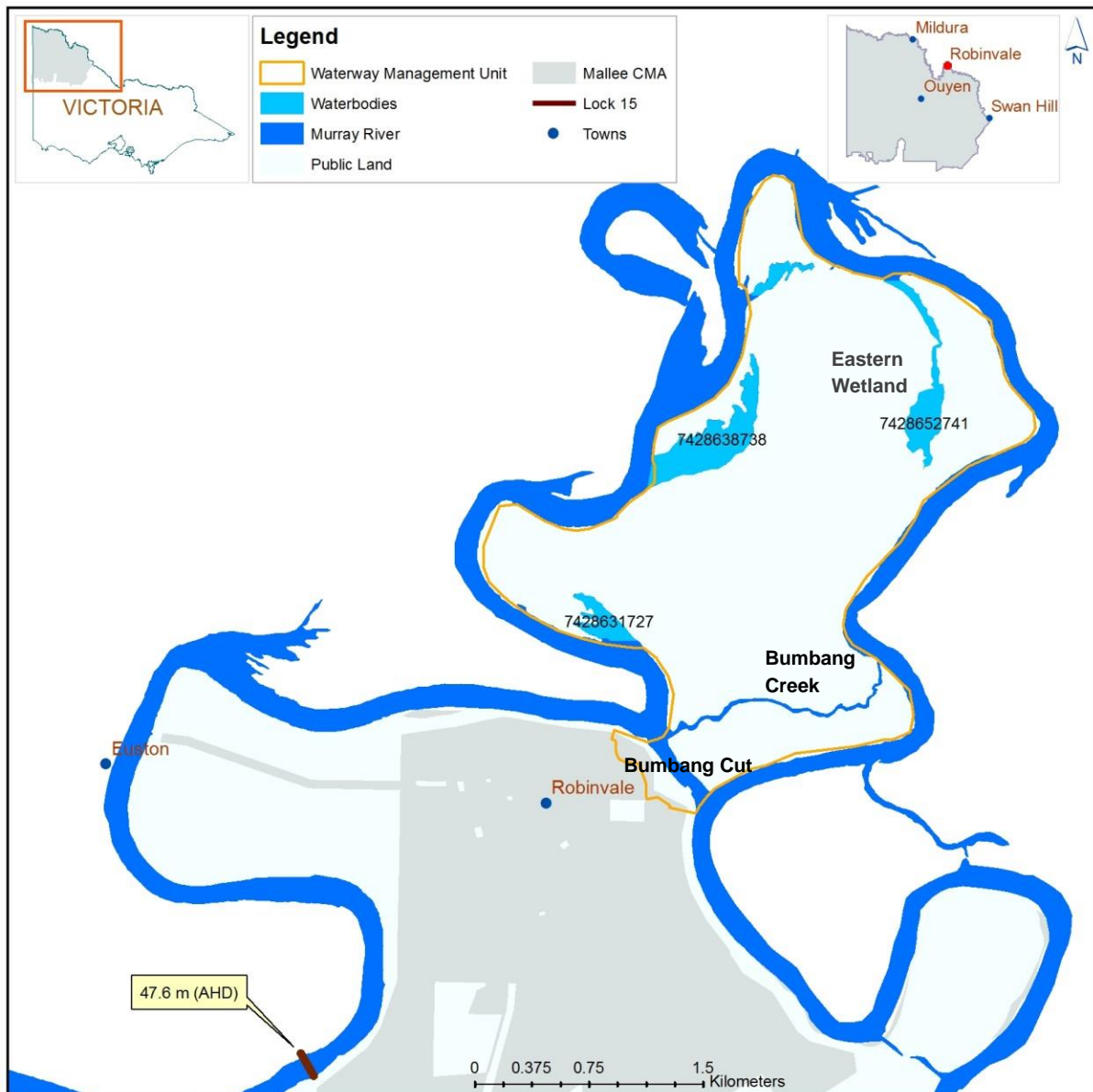
Figure 15. Inundation extent at baseline weir pool height (47.6 m AHD).
