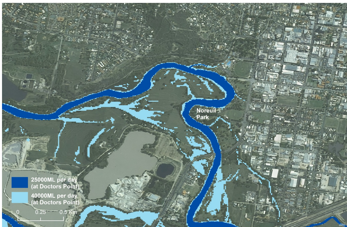
Figure 10: The inundation extent of flows of 25,000ML/day and 40,000ML/day as measured at Doctor's Point in Albury/Wodonga on the River Murray.
