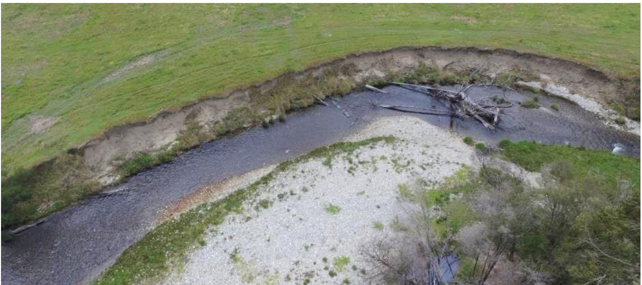
Figure 13. Accelerated meander migration following past removal of riparian vegetation.
